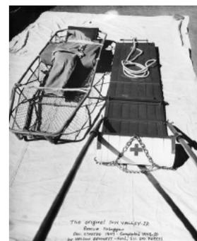
Using a Stokes litter on a lightweight toboggan, Nelson Bennett's sled used a chain for braking.
